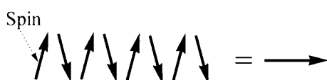
Fig. 4 Spin structure of canted antiferromagnets. Spontaneous magnetization grows to the right direction.
